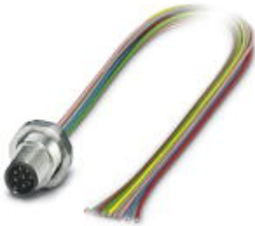
Sensor/actuator flush-type plug, 8-pos., M12, rear/screw mounting with Pg9 thread, with 0.5 m TPE litz wire, 8 x 0.25 mm², high-grade steel version
