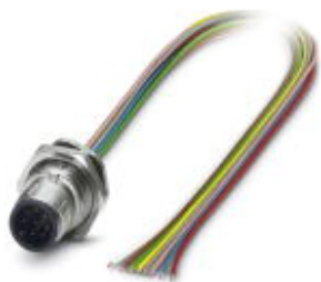
Sensor/actuator flush-type plug, 8-pos., M12-SPEEDCON, rear/screw mounting with Pg9 thread, with 0.5 m TPE litz wire, 8 x 0.25 mm 2
