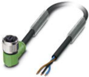
Sensor/Actuator cable, 3-position, PUR halogen-free, black-gray RAL 7021, free cable end, on Socket angled M12 SPEEDCON, A-coded, Cable length: 1.5 m
