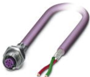
Bus system flush-type socket, PROFIBUS, 2-pos., M12, shielded, B-coded, rear/screw mounting with M16 thread, with 0.5 m bus cable, 2 x 0.25 mm 2
