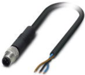
Sensor/Actuator cable, 3-position, PUR, black RAL 9005, Plug straight M5, A-coded, on free cable end, Cable length: 5 m
