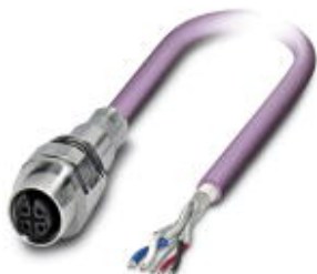
Bus system flush-type socket, DeviceNet/CANopen, 5-pos., M12, shielded, A-coded, front/screw mounting, with M16 thread, can be positioned, with 2 m bus cable, 2 x 0.2 mm 2 ; 2 x 0.32 mm 2
