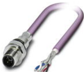
Bus system flush-type plug, DeviceNet/CANopen, 5-pos., M12, shielded, A-coded, front/screw mounting with M16 thread, with 2 m bus cable, 2 x 0.2 mm 2 , 2 x 0.32 mm 2
