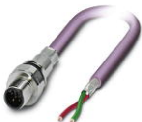
Bus system flush-type plug, PROFIBUS, 2-pos., M12, shielded, B-coded, front/screw mounting with M16 thread, with 1 m bus cable, 2 x 0.25 mm 2
