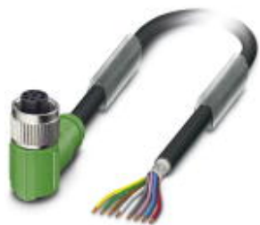
Sensor/Actuator cable, 8-position, PUR halogen-free, black-gray RAL 7021, shielded, free cable end, on Socket angled M12, A-coded, Cable length: 10 m
