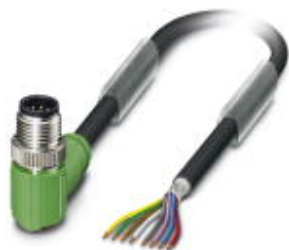
Sensor/Actuator cable, 8-position, PUR halogen-free, black-gray RAL 7021, shielded, Plug angled M12, A-coded, on free cable end, Cable length: 5 m
