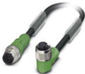
Sensor/Actuator cable, 8-position, PUR halogen-free, black-gray RAL 7021, Plug straight M12, A-coded, on Socket angled M12, A-coded, Cable length: 0.6 m
