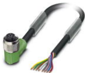
Sensor/Actuator cable, 8-position, PUR halogen-free, black-gray RAL 7021, free cable end, on Socket angled M12, A-coded, Cable length: 5 m
