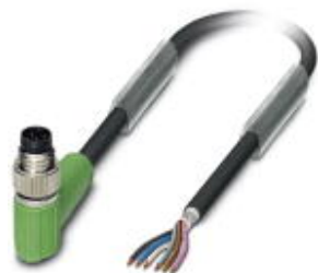
Sensor/Actuator cable, 6-position, PUR halogen-free, black-gray RAL 7021, shielded, Plug angled M8, on free cable end, Cable length: 5 m
