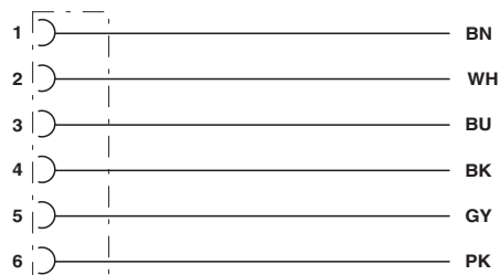
Contact assignment of M8 socket
