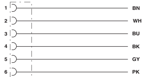
Contact assignment of M8 socket
