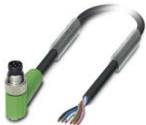
Sensor/Actuator cable, 6-position, PUR halogen-free, black-gray RAL 7021, Plug angled M8, on free cable end, Cable length: 1.5 m
