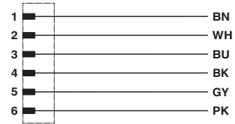
Contact assignment of the M8 plug
