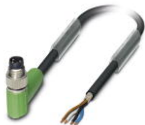
Sensor/Actuator cable, 4-position, PUR halogen-free, black-gray RAL 7021, shielded, Plug angled M8, on free cable end, Cable length: 5 m
