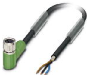
Sensor/Actuator cable, 3-position, PUR halogen-free, black-gray RAL 7021, shielded, free cable end, on Socket angled M8, Cable length: 3 m
