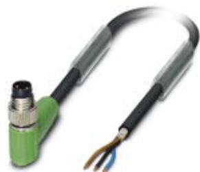
Sensor/Actuator cable, 3-position, PUR halogen-free, black-gray RAL 7021, shielded, Plug angled M8, on free cable end, Cable length: 1.5 m
