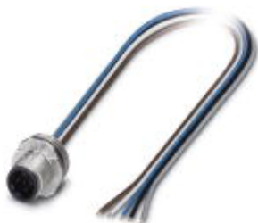
Fieldbus flush-type plug, INTERBUS/PROFIBUS, 5-pos., M12 SPEEDCON, B-coded, front/screw mounting with M16 thread, with 0.5 m TPE litz wire, 5x 0.34 mm 2
