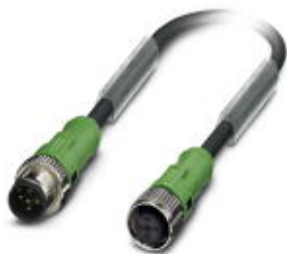
Sensor/Actuator cable, 5-position, PUR halogen-free, black-gray RAL 7021, Plug straight M12 SPEEDCON, A-coded, on Socket straight M12 SPEEDCON, A-coded, Cable length: 3 m
