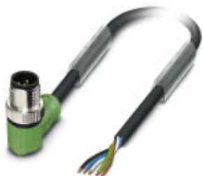
Sensor/Actuator cable, 5-position, PUR halogen-free, black-gray RAL 7021, Plug angled M12 SPEEDCON, A-coded, on free cable end, Cable length: 10 m
