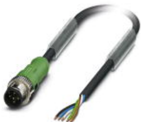
Sensor/Actuator cable, 5-position, PUR halogen-free, black-gray RAL 7021, Plug straight M12 SPEEDCON, A-coded, on free cable end, Cable length: 10 m
