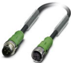
Sensor/Actuator cable, 4-position, PUR halogen-free, black-gray RAL 7021, Plug straight M12 SPEEDCON, A-coded, on Socket straight M12 SPEEDCON, A-coded, Cable length: 0.6 m
