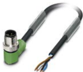
Sensor/Actuator cable, 4-position, PUR halogen-free, black-gray RAL 7021, Plug angled M12 SPEEDCON, A-coded, on free cable end, Cable length: 1.5 m
