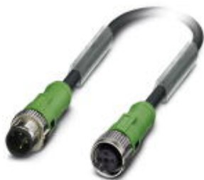
Sensor/Actuator cable, 3-position, PUR halogen-free, black-gray RAL 7021, Plug straight M12 SPEEDCON, A-coded, on Socket straight M12 SPEEDCON, A-coded, Cable length: 1.5 m
