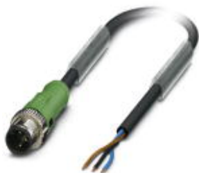
Sensor/Actuator cable, 3-position, PUR halogen-free, black-gray RAL 7021, Plug straight M12 SPEEDCON, A-coded, on free cable end, Cable length: 10 m
