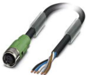
Sensor/Actuator cable, 5-position, PUR, black-gray RAL 7021, free cable end, on Socket straight M12 SPEEDCON, A-coded, Cable length: 5 m
