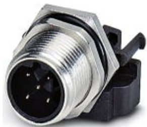
Sensor/Actuator flush-type plug, 5-pos., M12, B-coded, rear/screw mounting with M12 thread, with straight solder connection
