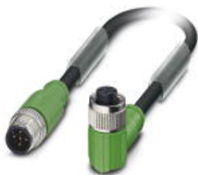
Sensor/Actuator cable, 5-position, PUR halogen-free, black-gray RAL 7021, shielded, Plug straight M12, A-coded, on Socket angled M12, A-coded, Cable length: 0.6 m
