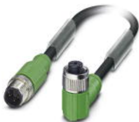
Sensor/Actuator cable, 4-position, PUR halogen-free, black-gray RAL 7021, shielded, Plug straight M12, A-coded, on Socket angled M12, A-coded, Cable length: 3 m
