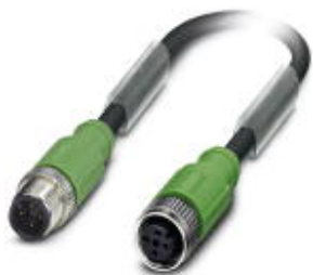
Sensor/Actuator cable, 4-position, PUR halogen-free, black-gray RAL 7021, shielded, Plug straight M12, A-coded, on Socket straight M12, A-coded, Cable length: 0.6 m
