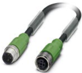
Sensor/Actuator cable, 3-position, PUR halogen-free, black-gray RAL 7021, shielded, Plug straight M12, A-coded, on Socket straight M12, A-coded, Cable length: 0.6 m
