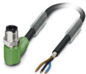
Sensor/Actuator cable, 3-position, PUR halogen-free, black-gray RAL 7021, shielded, Plug angled M12, A-coded, on free cable end, Cable length: 10 m
