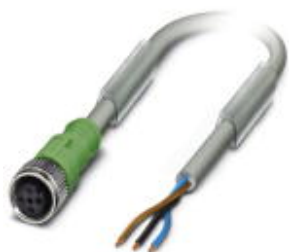
Sensor/Actuator cable, 3-position, PUR halogen-free, welding sputter-resistant, highly flexible, gray RAL 7001, free cable end, on Socket straight M12, A-coded, Cable length: 10 m, for robots and drag chains
