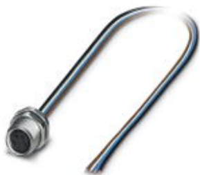
Sensor/actuator flush-type socket, 4-pos., M8, rear/screw mounting with M10 thread, with 0.5 m TPE litz wire, 4 x 0.25 mm 2
