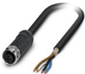
Sensor/Actuator cable, 4-position, PE-X/PE-X halogen-free, black-gray RAL 7021, shielded, free cable end, on Socket straight M12, A-coded, Cable length: 2 m, for outdoor applications, With high-grade steel knurl
