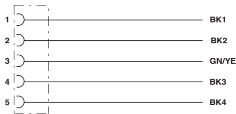
Contact assignment of 7/8" socket
