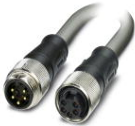
Power cable, 5-position, PVC, gray RAL 7001, Plug straight 7/8"-16UNF, A-coded, on Socket straight 7/8"-16UNF, A-coded, Cable length: 0.6 m, 1.5 mm 2 conductor cross section, For power supply
