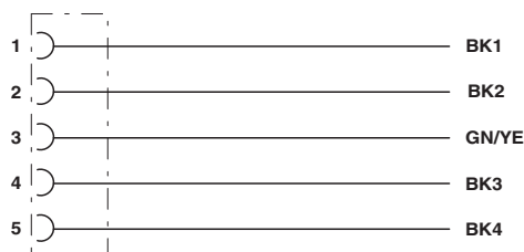
Contact assignment of 7/8" socket
