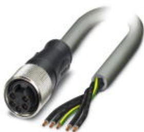
Power cable, 5-position, PVC, gray RAL 7001, free cable end, on Socket straight 7/8"-16UNF, Cable length: 10 m, 1.5 mm 2 conductor cross section, For power supply
