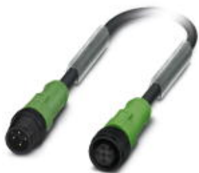
Sensor/Actuator cable, 4-position, PUR halogen-free, black-gray RAL 7021, Plug straight M12, A-coded, on Socket straight M12, A-coded, Cable length: 1.5 m, with plastic knurl
