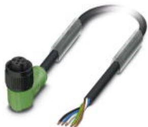
Sensor/Actuator cable, 5-position, PUR halogen-free, black-gray RAL 7021, free cable end, on Socket angled M12, A-coded, Cable length: 3 m, with plastic knurl
