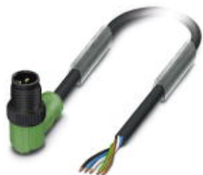
Sensor/Actuator cable, 5-position, PUR halogen-free, black-gray RAL 7021, Plug angled M12, A-coded, on free cable end, Cable length: 10 m, with plastic knurl
