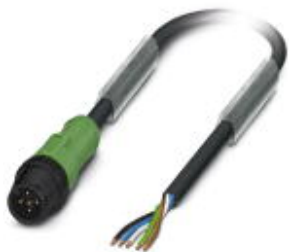
Sensor/Actuator cable, 5-position, PUR halogen-free, black-gray RAL 7021, Plug straight M12, A-coded, on free cable end, Cable length: 10 m, with plastic knurl
