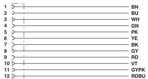
Contact assignment of the M12 socket
