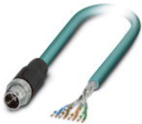
Assembled Ethernet cable, CAT6 A , shielded, 4-pair, AWG 26 stranded (7-wire), RAL 5021 (water blue), M12 plug on free conductor end, length 1 m
