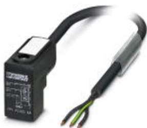
Sensor/Actuator cable, 3-position, PVC, black RAL 9005, free cable end, on Valve connector CI (9.4 mm), with 1 LED, connected with Z diode, Cable length: 1.5 m
