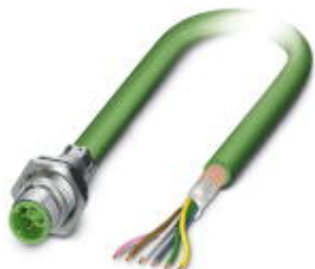
Bus system flush-type plug, INTERBUS, 5-pos., M12, shielded, B-coded, SPEEDCON, rear/screw mounting with Pg9 thread, with 5.0 m bus cable, 3 x 2 x 0.25 mm 2
